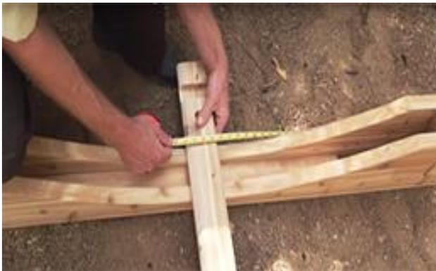
Center the stave onto the cradle and measure 5 ½" (14cm) from the end of the stave to the edge of the cradle.
