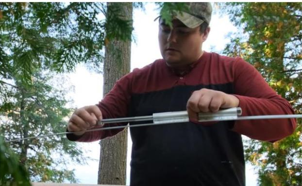
Pre-assemble the front and back bands and thread the nut on just enough to hold it together.
