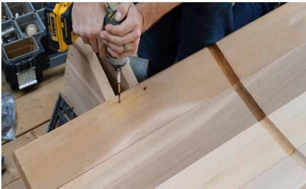
Place 2- 2 ½" (64mm) screws into the 3<sup>rd</sup> stave on either side lining up with the cradle underneath.
